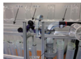
Compact traveling robot continuously measures waste heat boiler water pipe thickness and laboratory test equipment
