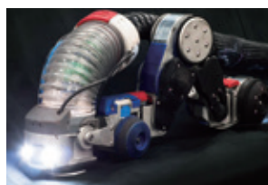
Compact traveling robot continuously measures waste heat boiler water pipe thickness and laboratory test equipment
