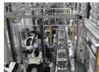
Automated dry vacuum pump assembly line
